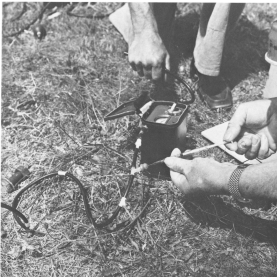
Fig. 6. Portable detector 'A' showing sampling method.
