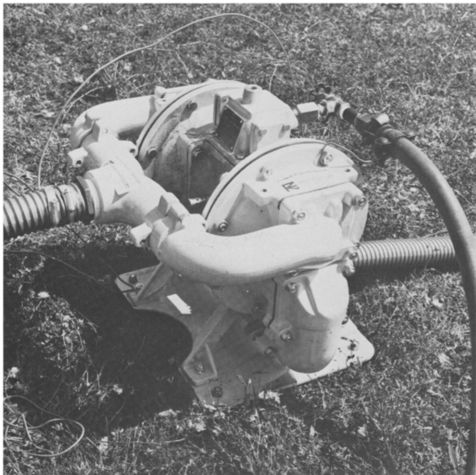
Fig. 5. Compressed-air operated portable pump.
